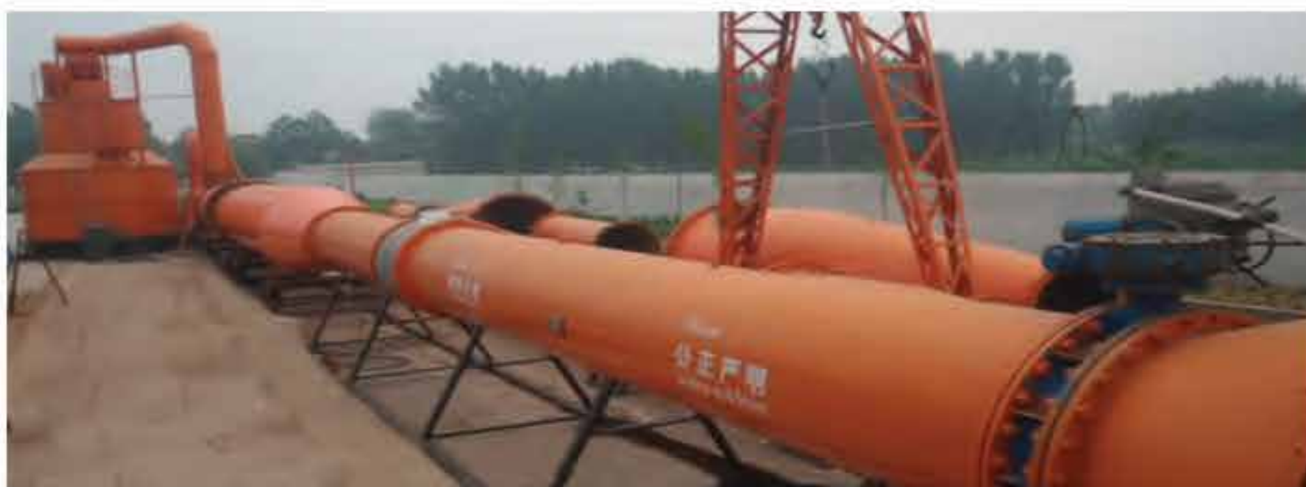
DN800 ~DN3000 Liquid Flow Meter Calibration Device
