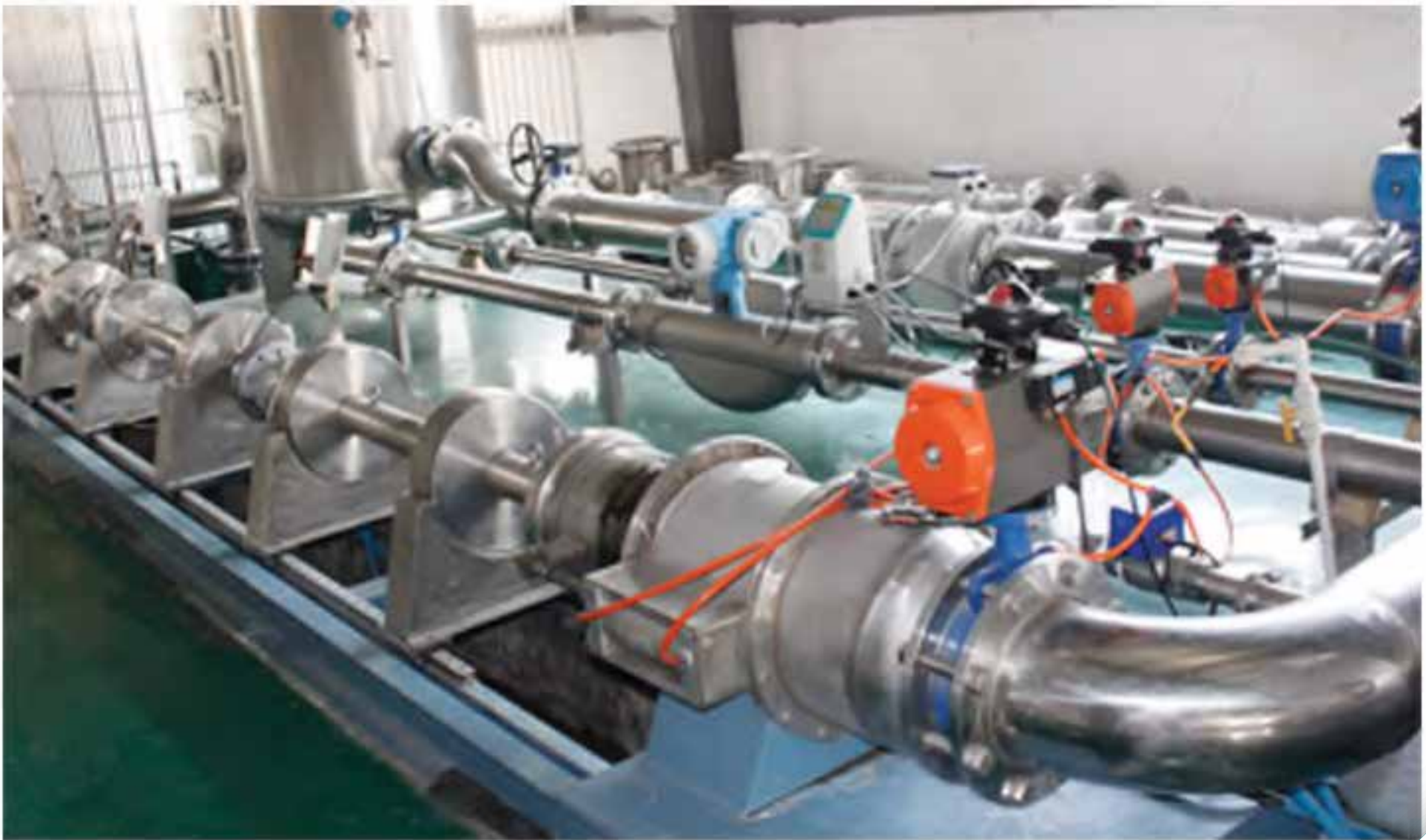
DN65-DN300 Standard Meter Liquid Flow Meter Calibration Device
