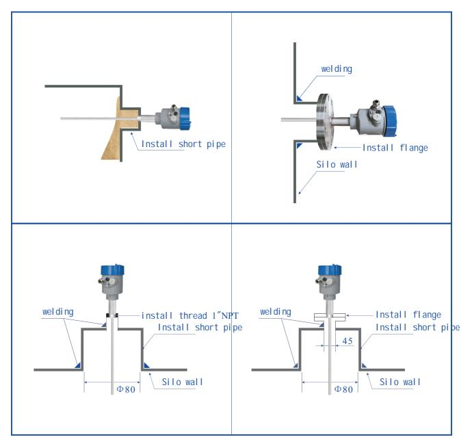
Note: When installing the tuning fork level switch horizontally, the length G of the probe protective sleeve must extend into the container wall. When installing vertically, the total length S of the probe must be equal to or greater than the position of the control point.
